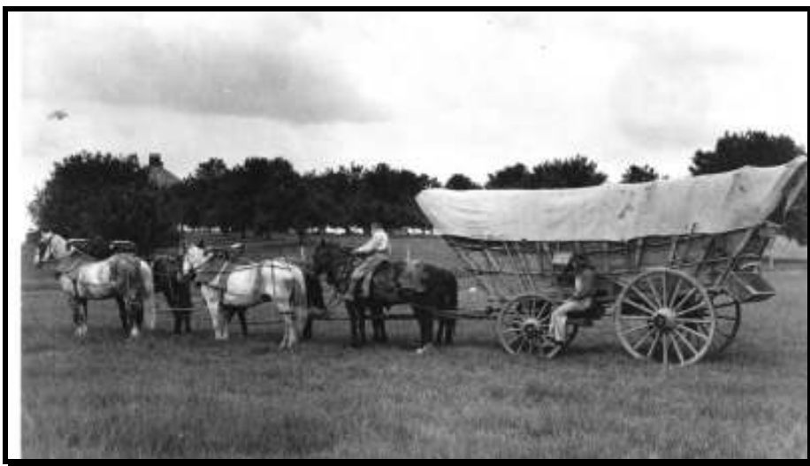
A Conestoga wagon used by pioneers in the 1700-1800s. Notice there is no buckboard in front of the wagon for the driver to sit – he either sat on a horse, walked along side, or used the “lazy board” located where the man is sitting on the side of the wagon.
